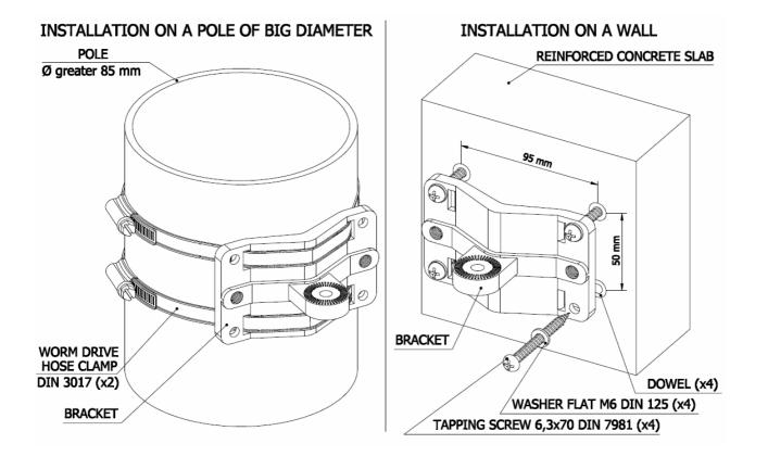
**Attention! MOUNT-KIT-85 does NOT contain worm drive hose clamps** or other additional fixtures used in possible variants of installation.
