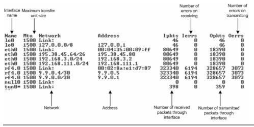
If the interface has several aliases the statistics is still measured for physical interface in a whole. For example, see rf4.0 or eth0 interfaces above. The numbers shown in 4 right columns correspond in physical interface.
