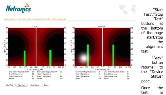
started antenna alignment can be monitored using graphical and text indicators. Indicators for both local and remote devices are displayed together on the same page that allows viewing the alignment process for both sides of the link.
