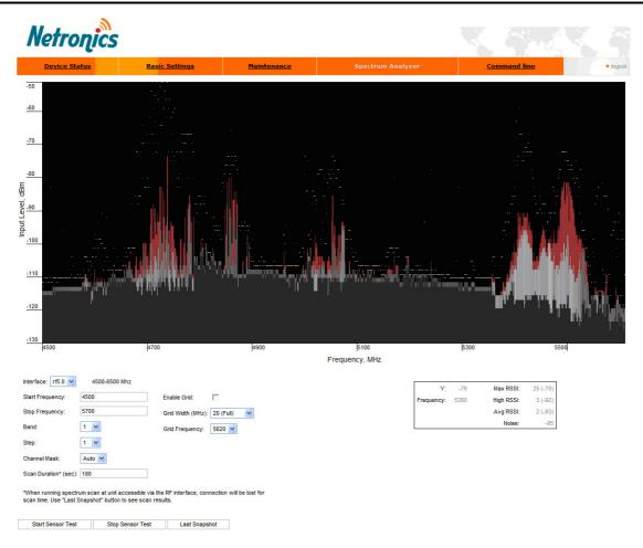
«Spectrum Analyzer» tab provides deep analysis of radio emission sources. In this mode device scans the radio spectrum on all available frequencies. To obtain information as complete as possible, the scanning process may take some time.
