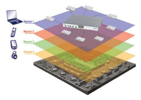
NetGlide channel blanket deployment of APs permits 'n' and legacy 'a/b/g' devices to co-exist, in either band, with full speed and throughput maintained for all.
